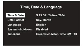
2. The 'Time & Date' option will be highlighted use the ⇒ button or the keyboard joystick to move to the hours setting.
